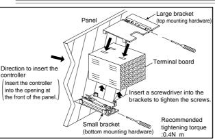
After opening the mounting hole on the panel, follow the procedures below to install the controller:
