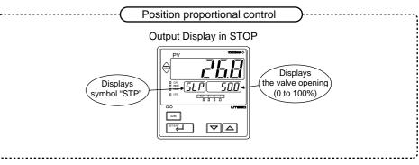
\* Switching the target setpoint number (SPN) in STOP allows any preset output value (n.PO) to be switched.
